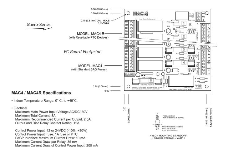
Connections: Captive Screw Terminals for #14 to #22AWG Wire PTC Outputs: 2.5A PTC Resettable Devices included (MAC4R) Fuse Outputs: 2.0A 3AG-type Fuses included (MAC4)
