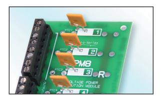
A PTC is usually soldered into a circuit board. It cannot be replaced quickly. In a distributed power system with PTCs, detecting which circuit is tripped can be troublesome and there are no visual clues. The device cannot be removed or turned off to enable modifications to the protected circuit. To enable this, the power source to the PTC must be turned off
